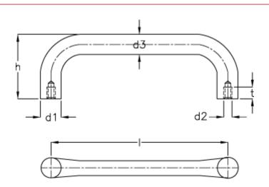
$\begin{array}{ll} d1 &= 20 \\ d2 &= M8 \\ d3 &= 14 \\ h &= 47 \\ I &= 112 \\ t \mbox{ min} = 15 \end{array}$
